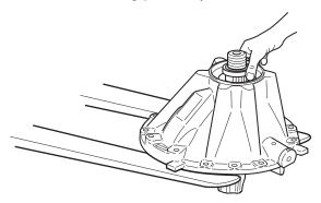
7. Install the outer bearing cone.
