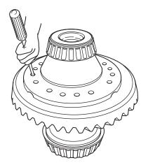
9. Install the ring gear capscrews.
