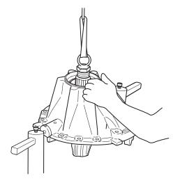
14. Install the drive yoke and pinion nut.
