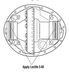
12. Install the carrier differential bearing caps and capscrews. Make certain there is no gap between the carrier cap and the carrier surface.
