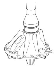
**Note:** If a press is not available, use a sleeve or bearing driver and a hammer to install the cups.
