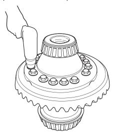
11. Lower assembled differential assembly in to the carrier using a hoist and a strap. Be careful not to damage the differential bearings lowering the assembly.
