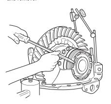
9. Using a chain hoist and the proper strap, lift the ring gear and wheel differential assembly from the carrier.
