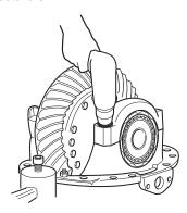
14. Recheck the backlash. For new gearing, the backlash should be between 0.008" and 0.018" (0.20 and 0.46 mm).
