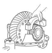
7. Use an impact gun to snug all carrier cap fasteners.
