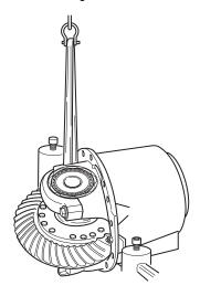
15. Use the correct socket and a breaker bar to rotate the differential. The differential should be hard to turn. Rotate the pinion until the ring gear rotates 3 or 4 times in both directions.
