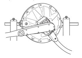
16. Use an in. lbs. torque wrench and correct socket to check the rolling torque of the pinion. Read torque while rotating the assembly. Record the rotating torque, not the breakaway torque. Torque must be between 20 to 50 lbs. in. If the torque recorded is not within the specified torque, the pinion spacer must be changed. Repeat Steps 6-17.
