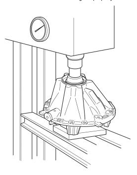
12. With 5 tons of force on the press, you should be able to feel a small amount of drag from the bearing as you rotate the carrier. If the carrier turns with no drag at all, the pinion spacer thickness should be decreased by using a thinner spacer. If the carrier is hard to turn, the spacer thickness must be increased.
