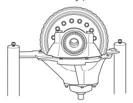
**Note:** For easier disassembly, loosen but do not remove the pinion nut.
