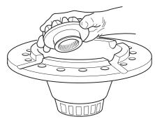
4. Assemble the side pinions and thrust washers onto the wheel differential spider. Apply a thin coat of oil to the mating surfaces of the side pinion and differential spider. Install the wheel differential nest on top of the side gear
