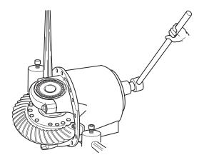
22. When contact pattern is correct, use a punch with a round head to stake the threaded bearing cups in place. Stake the outer edge of the bearing adjustment ring into the machined slots in the carrier bearing bore on both sides. Must be staked at two locations. Rotate cup if necessary to provide surfaces for staking.
