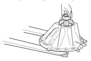
9. Align a 6" x 6" x 6" wood block under the drive pinion, then lower the carrier and pinion assembly into a press so that it is supported by the block.
