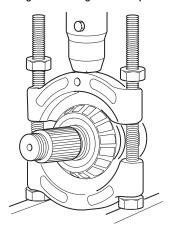
Mount the puller horizontally to press the bearing from the pinion.
