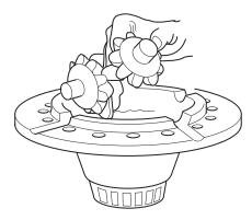
5. Install the flange half side gear and thrust washer.
