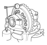
Measure the ring gear total backface runout. Indicator reading should not exceed 0.010" (0.25 mm).
