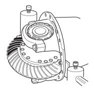
13. Make a sling out of a strap and position around the plain half of the wheel differential.
