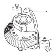
19. Make a sling out of a strap and position around the plain half of the wheel differential.
