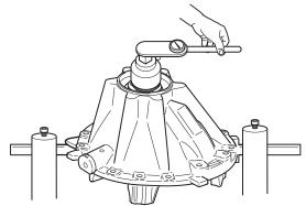
17. Now remove the pinion nut and yoke and install the pinion seal. Use Spicer's seal drive (part number 210749) and drive adapter (part number 131472).
