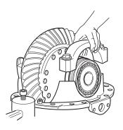
13. Use an impact gun to snug all carrier cap fasteners.
