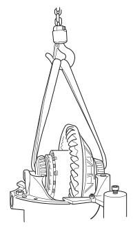
12. Install the bearing cup and bearing adjuster to the flange half side first.
