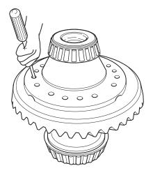
9. Install the ring gear capscrews.
