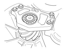
**TIP:** If you are unable to torque the yoke nut correctly, try torquing the nut with the truck wheels on the ground and with the axle shafts installed.
