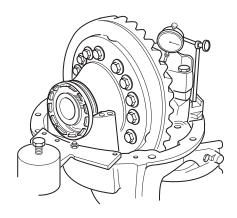
6. Install the carrier differential bearing caps and capscrews. Make certain there is no gap between the carrier cap and the carrier surface.
