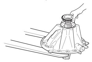
8. Install a pinion nut finger tight. This will hold the pinion in place while it is positioned into the press.
