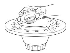
4. Assemble the side pinions onto the wheel differential spider. Apply a thin coat of oil to the mating surfaces of the side pinion and differential spider. Install the wheel differential nest on top of the side gear.
