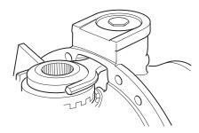
Remove the threaded cylinder cap.
