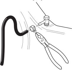
Push hose firmly against fitting. Rotate hose to point down.
