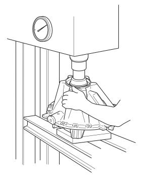
13. Remove the carrier from the press. Secure the carrier in a head stand.
