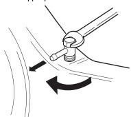
Plastic only: Tighten until one thread is showing.
