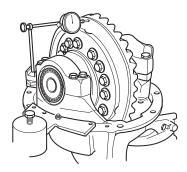
Measure the ring gear total backface runout. Indicator reading should not exceed 0.010" (0.25 mm).
