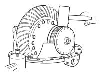
With a dial indicator, check the ring and pinion backlash. Set the backlash from 0.010" to 0.012". This will give you room to adjust the contact pattern, if necessary.
