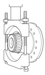
b. Mount the puller horizontally to remove the cone.
