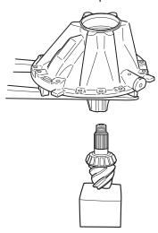
Install the pinion spacer.
