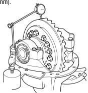
11. Check the ring gear tooth pattern. Paint 5 or 6 ring gear teeth 180 degrees apart on the ring gear.
