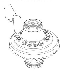
Remove the flange half differential case and bearing assembly. Use a screwdriver at the spider arm machined slots of the case to loosen the flange from the ring gear.
