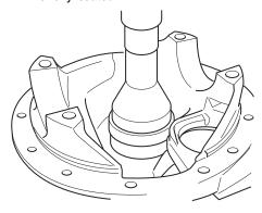
c. If replacement of the output shaft side gear bearing cup is necessary, use either of the following methods:
