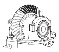
18. With the carrier mounted in a head stand, roll the carrier on its side.
