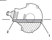
1 - Oil Filler Hole 2 - Lost Oil Capacity
