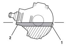
1 - Oil Filler Hole 2 - Lost Oil Capacity
