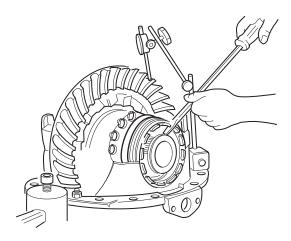
Tighten the plain half adjuster two lug notches. Start with the notch at the top, count two notches counterclockwise on the adjuster so that the notch is facing straight up. You now have a two notch preload.
