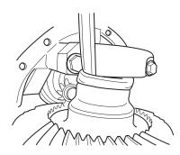
14. Connect the end of the strap to a hoist and apply pressure to the sling.
