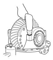
8. Recheck the backlash. For new gearing, the backlash should be between 0.008" and 0.018" (0.20 and 0.46 mm).
