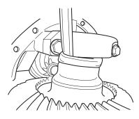
20. Connect the end of the strap to a hoist and apply pressure to the sling.
