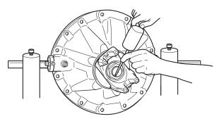
To de-stake the nut, use a chisel or drift with a round tip. The flange of the nut must be pushed far enough outward so that the staked area will not interfere with the pinion threads when the nut is removed. See diagram below.
