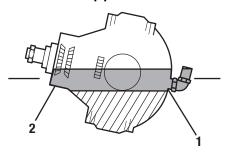
1 - Oil Filler Hole 2 - Additional Oil Capacity
