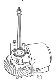
21. Use the correct socket and a breaker bar to rotate the differential. The differential should be hard to turn. Rotate the pinion until the ring gear rotates 3 or 4 times in both directions. See page 30, "Adjust Tooth Contact Position" for descriptions of correct pattern position for new and used gearing.
