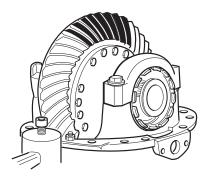
12. With the carrier mounted in a head stand, roll the carrier on its side.
