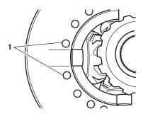
1 - Match spacing of holes on each side of spider slots
